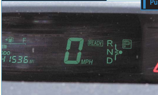
Figure 4. The "READY" light on the dash. Anytime this light is on, a Prius can start at any time!
