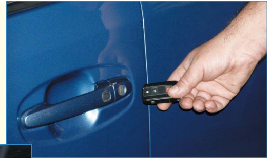
Figure 2. The "Smart Key" transponder.
