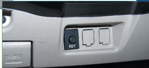
Figure 5. The Smart Key Disable button. Pushing the button "in" will disable the system.
